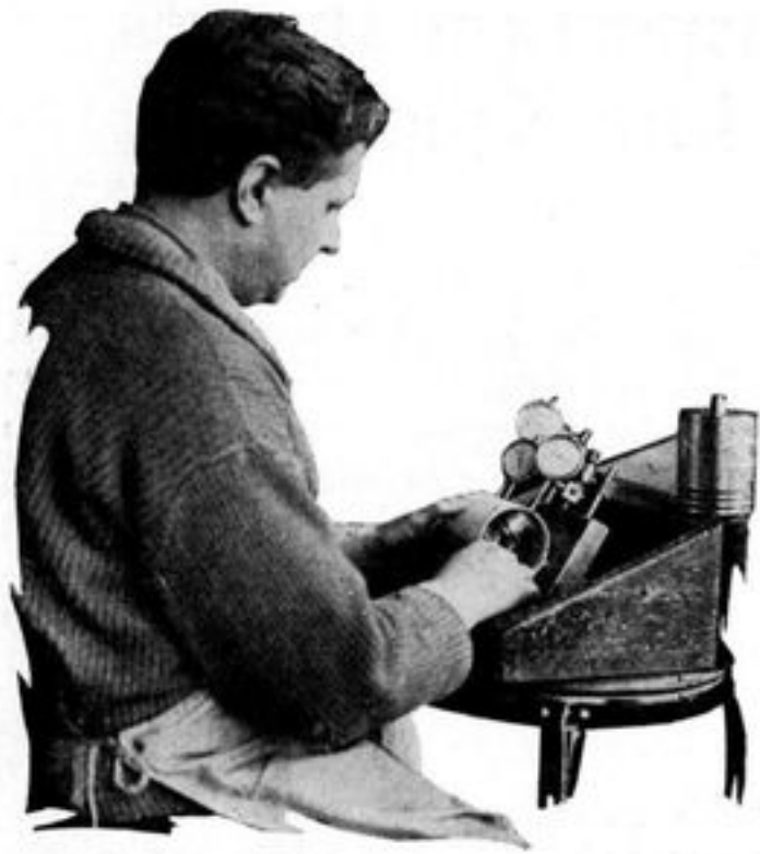
The indicator gauge, which determines the acceptance of Franklin pistons, checks for all dimensions.
